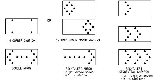
5. The "CAUTION" display consists of four corner lamps flashing simultaneously, or the Alternating Diamond Caution mode as shown.
